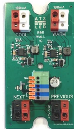
AL-R@R Wall - Temporary Switch
